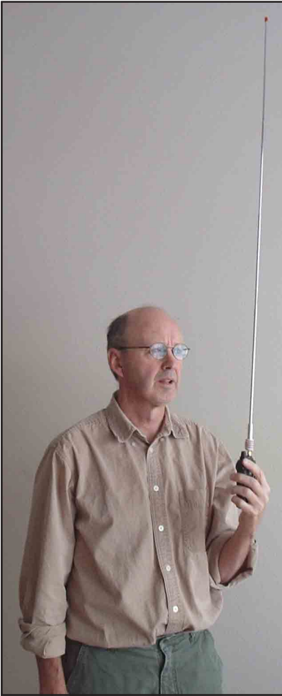
Fig 1—Author with hand-held and homebrew 2-m half-wave antenna.
