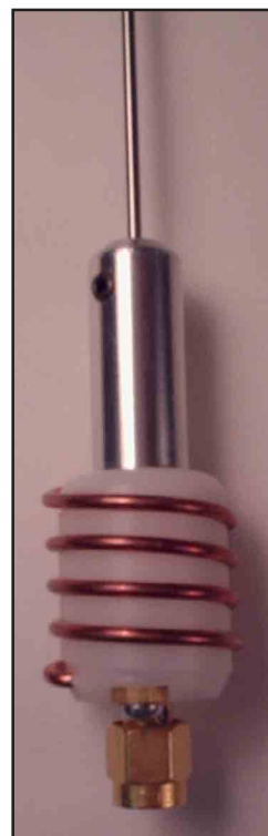
Fig 14— 2 meter matching network with the wire element.
