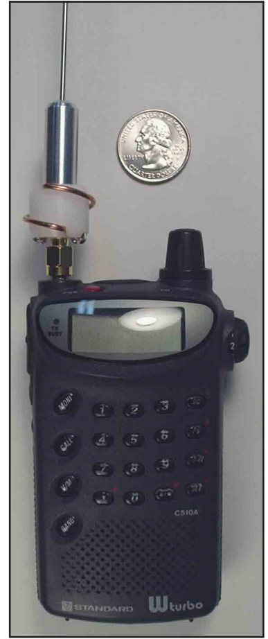
Fig 3—A hand-held with a KØDK 70 cm half-wave whip antenna.
