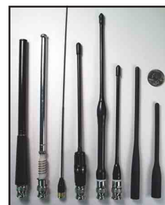
Fig 15—The hand-held antennas used for measurement comparisons to the homebrew half-wave antennas for 2 meters and 70 cm. In order from the left—Larsen telescoping half-wave, AEA telescoping half-wave, Pryme quarter wave whip, Standard dual band for C510A, Larsen 2M, Larsen 70cm, Icom dual band for IC-Q7A, Standard dual band for C528A.
