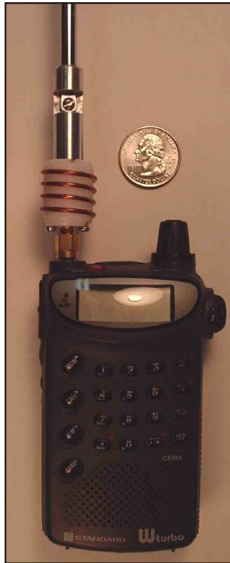
Fig 2—A hand-held with a KØDK 2-meter half-wave telescoping antenna.
