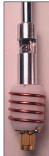
Fig 9—Matching network for 2-meter end-fed half-wave, telescoping element version.
